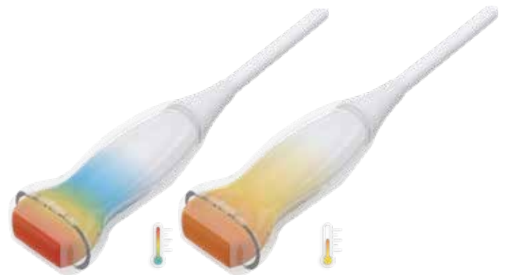
Fig. 4 - Thermal behavior of the probe without (left) and with (right) thermal efficiency technology. In both cases, the amount of heat does not exceed that allowed by the standards. Nevertheless, due to the lower temperature of the probe surface, the PX 1-5 delivers higher transmit and receive sensitivity and therefore produces a higher quality image and Doppler signal.
